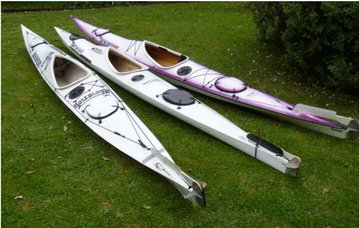
Roger's Barracuda fleet. Left to right B1 The original, B2 The Bullet, B3 The Kevlar Discovery. All kayaks are 5.8 metres long. B1 and B3 have a 520mm beam and the Bullet is 470mm and weighs 18kgs.
