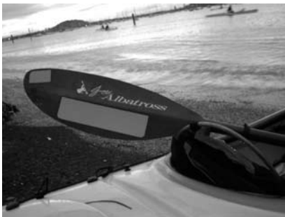
Red reflective tape on the front of a black carbon paddle blade. The rear of this blade also has tape attached.
