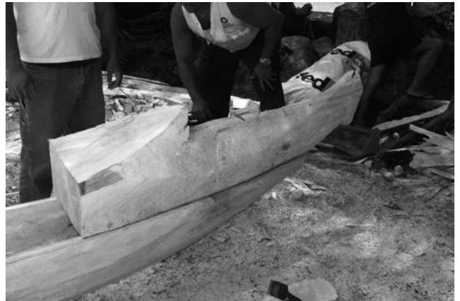
Fitting the stern section
