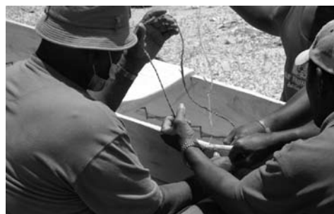
Stitching and lashing the components together
