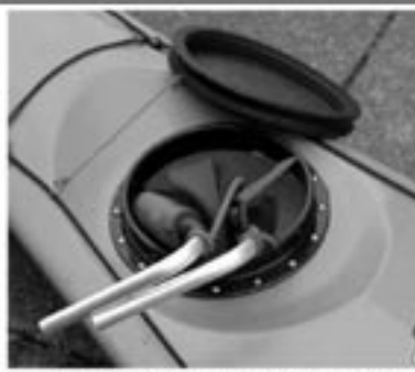
Frame stored through 180 mm hatch
